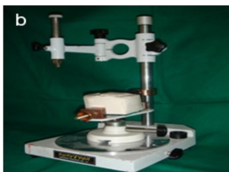
[Table/Fig-4b]: Plaster Index Placed on Surveying Table
